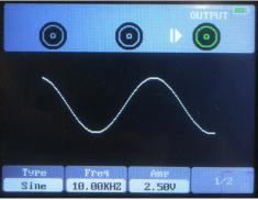
**6.** Press button, the backlight of the button turns green, i.e. output sine waveform.
