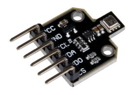
The BME680 is the new, compact ambient sensor with integrated sensor technology for humidity, pressure, temperature and air quality.
