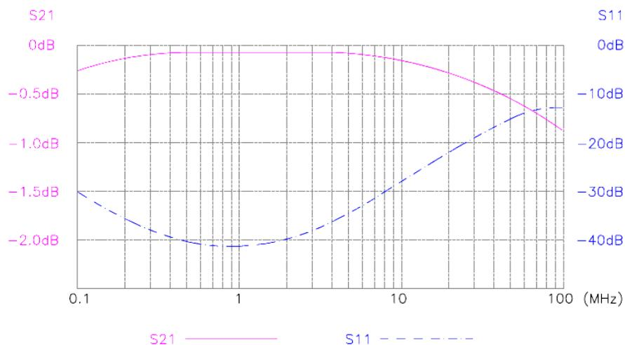
The MI 1005 is characterized by Return Losses of more than -10db at frequencies of 100 MHz and a low insertion loss of less than -1,1 dB.
