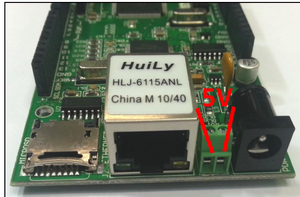
Fig. 2. Supplying 5V directly. [Fornire 5V diretti]
