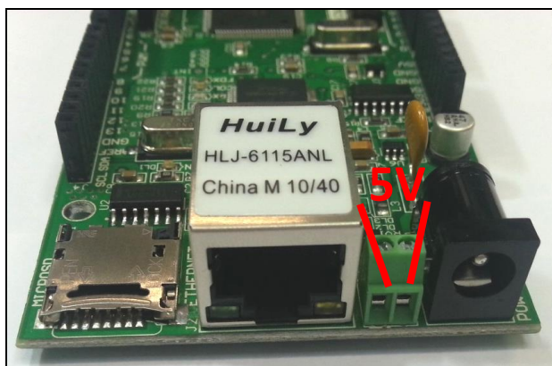
Fig. 2. Supplying 5V directly. [Fornire 5V diretti]
