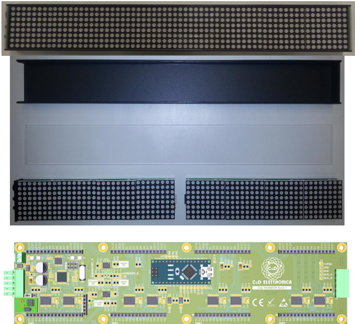
Fig. 3. Cased 2-cell FlashMat display, with an Arduino Nano master board (optional) installed on one of the cells.
