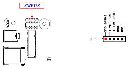
\*Note: Maximum current limit is 0.3A while using 5V working voltage.
