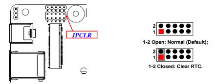
Pin (3-4) of JPCLR (10-pin)): Clear CMOS (2.0 pitch)
