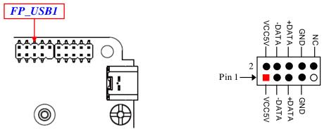
\*Note: Maximum current limit is 0.5A while using 5V working voltage
