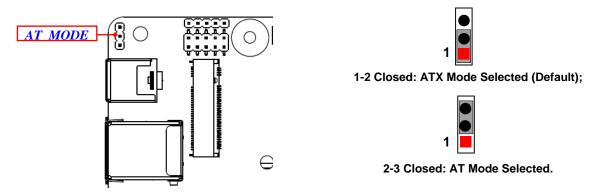
\*ATX Mode Selected: Press power button to power on after power input ready; AT Mode Selected: Directly power on as power input ready.
