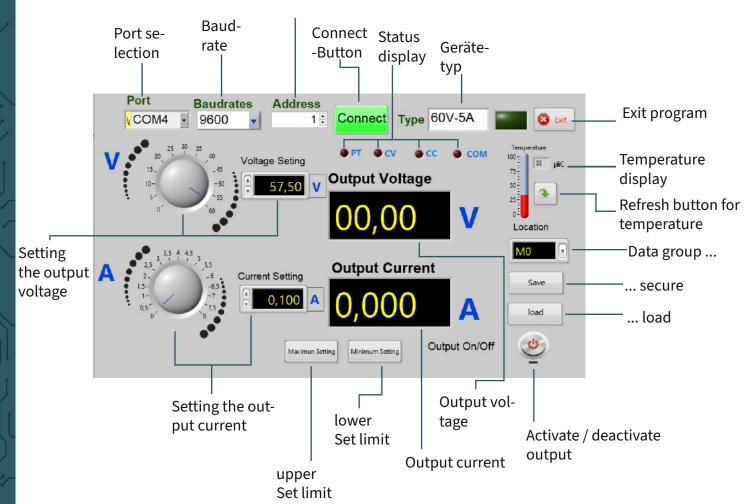
The output is deactivated when the button is displayed in red. It turns green as soon as it is activated.
