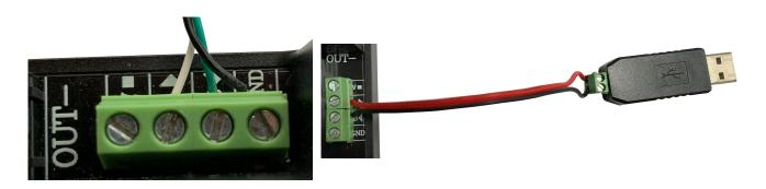
Once the cables have been connected to the power supply unit in accordance with the instructions in the image and table, connect the device to the PC via USB. in the Device Manager under "Ports (COM & LPT)", check which port the power supply unit is connected to; in this example it would be COM4.
