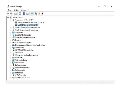
You must now install drivers to enable communication between the power supply unit and the PC . To do this, you can use the NI-VISA software, which you can download here which you can download here.
