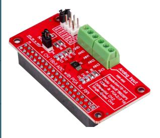
With the help of the RB-ADC01 you can read analog data with your Raspberry Pi. The 16-bit chip ADS1115 is an analog to digital converter that processes the analog signal to digital data and sends it via I2C bus to the Raspberry Pi.
