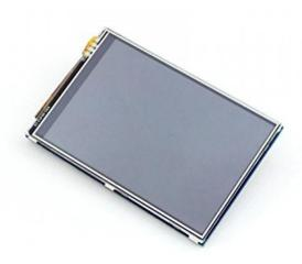
With the 3.5 Inch TFT Touchscreen-Display you can easily build a Mini-Tablet-PC based on an Raspberry Pi. The display, with a maximum resolution of 480x320 pixels, can be attached to the GPIO connections so that you won't need any mounting-skills.
