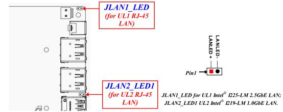
\*Note: Maximum current limit is **300uA** while using **3.3V** working voltage.
