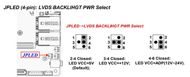
\*Note: Maximum current limit is 2A while using 5V or 12V.
