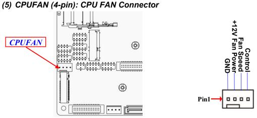
\*Note: Maximum current limit is **1.5A** while using 12V working voltage.
