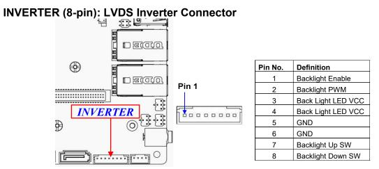
\*Note: Maximum current limit is 2A while using 5V or 12V or adapter DCIN Voltage(12V~24V).
