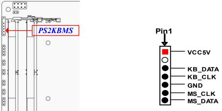
\*Note: Maximum current limit is 500mA while using 5V working voltage.
