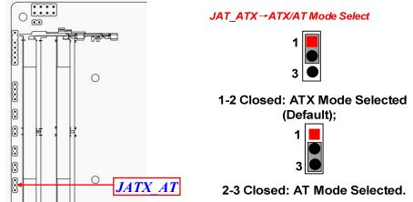
\*ATX Mode Selected: Press power button to power on after power input ready; AT Mode Selected: Directly power on as power input ready. Pin (1-2) of JBAT (4-pin): Clear CMOS Settings
