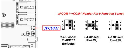
\*Note:Maximum current limit is 500mA while using 5V or 12V.
