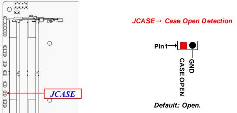
**Pin 1-2 Short**: When Case open function pin short to GND, the Case open function was detected. When Used, needs to enter BIOS and enable 'Case Open Detect' function. In this case if your case is removed, next time when you restart your computer, a message will be displayed on screen to inform you of this.
