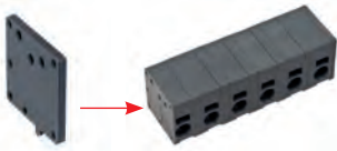
Side Wall with Coding Pin SW-AK4200-CP-H-baGY Article Number: 5420000002 The sidewall with coding pin (SW-CP) ensures the right assembly of the terminal block in the PCB. The coding pin thereby is inserted into the corresponding PCB hole. The SW-CP substitutes the standard side wall (SW).
